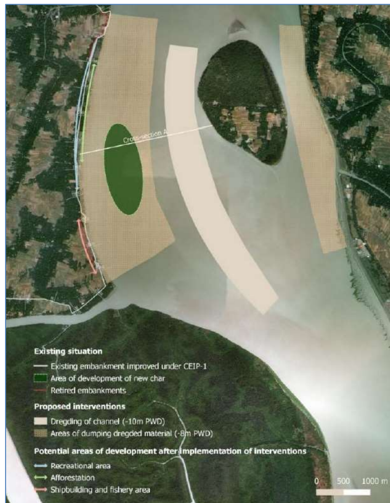
Figure 3-9: Layout of intervention in Polder 35/1: dredging of channel and deposition at the erosion hotspot 45
